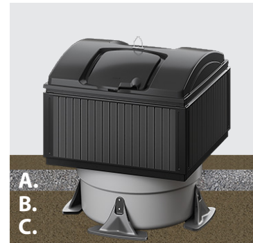
Image 2. Filling the pit A. Finishing layer, 100 mm B. Anchoring layer, gravel 0/32, 400 mm C. Levelling layer, crushed gravel 0/16, min. 50 mm
