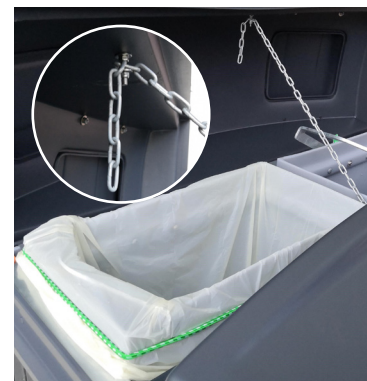
Image 5. Installation of the side hinge
